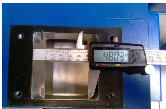
View of inlet size of CM100 = 48mm
