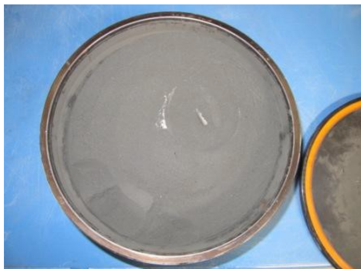
Grinding result after 2 minutes / 95%<200 micron
