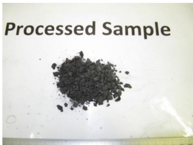
Sample was pre-crushed with the LMC100D Jaw Crusher Down to 3 mm.
