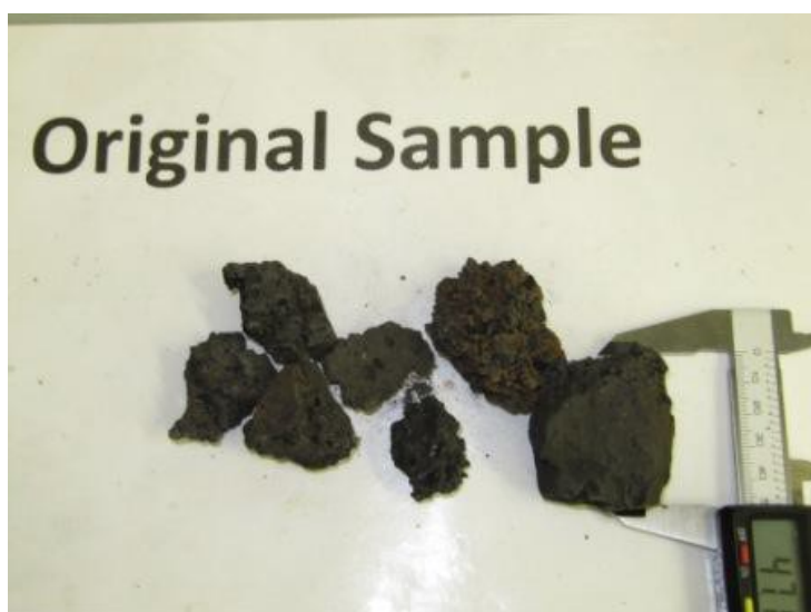
Original sample material with feed size of up to 48mm
