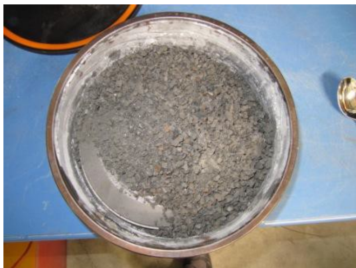
Loading the 2000ml bowls with 2 kgs of pre-crushed lead
