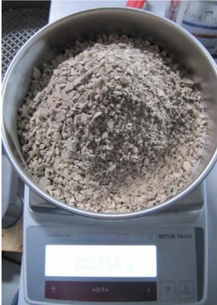
Original sample No 1. Limestone (Feed Size of up to 15mm) quantity of 1008,57 gram
