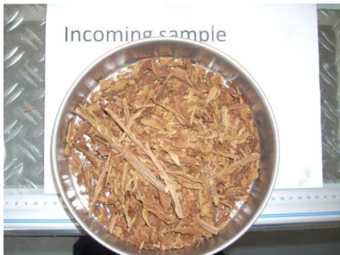
Original sample material with feed size of up to 102,70 mm
