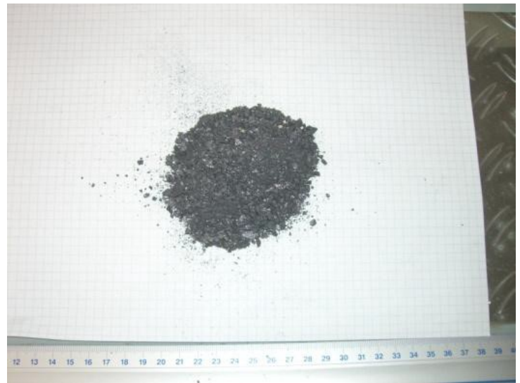
3mm after pre-crushing with LMFC250 Fine Crusher
