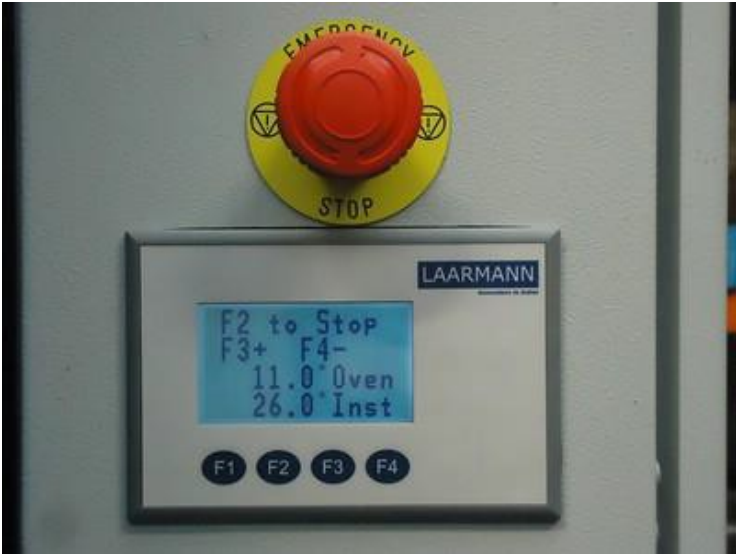
Press F2 to Stop Press F3 to increase and F4 to decrease the temperature
