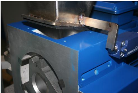
Safety switch hopper lid.
