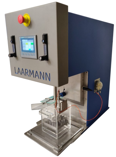
Flotation machine with temperature meter
