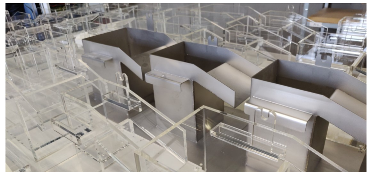
acrylic and stainless steel flotation cells in various volumes
