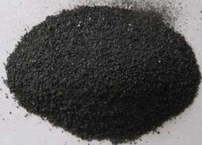
Processed sample / Fine-Cutting with 2,00mm Sieve
