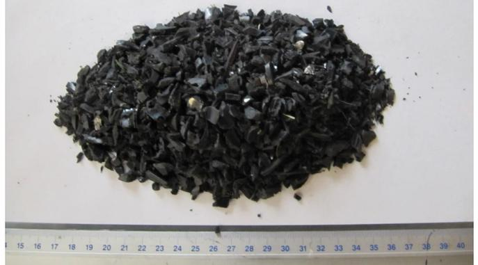
Processed sample / Pre-Cutting with 12,00mm Sieve
