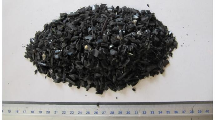
Processed sample / Pre-Cutting with 12,00mm Sieve
