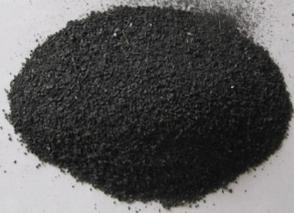
Processed sample / Fine-Cutting with 2,00mm Sieve
