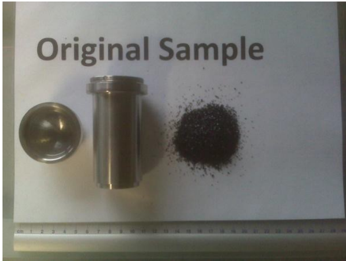
Original sample No 1. Glasfibres (Feed Size of up to 3mm)
