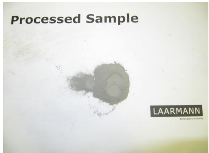
Result after 2 minutes of dry grinding about 30 \mu m
