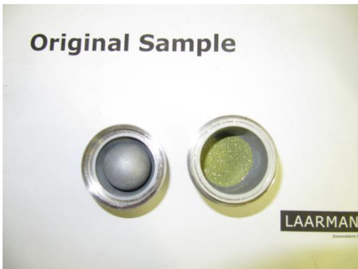
Amount loaded to the Mill 20 grs. Grinding time about 2 minutes.
