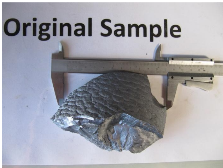
Picture 1) Original sample Polysilicon (Feed Size of up to 120mm)
